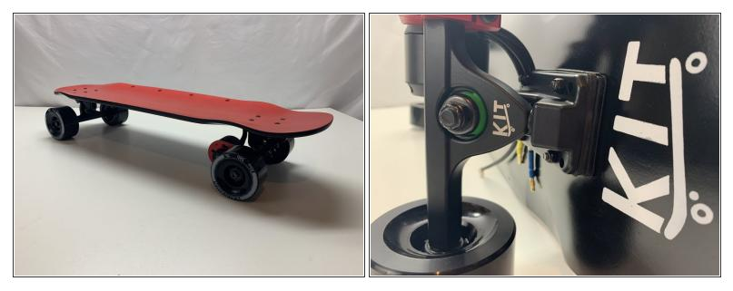
Install the drivetrain on the rear of the deck. Use one riser and 4x M5x35 bolts and locknuts
