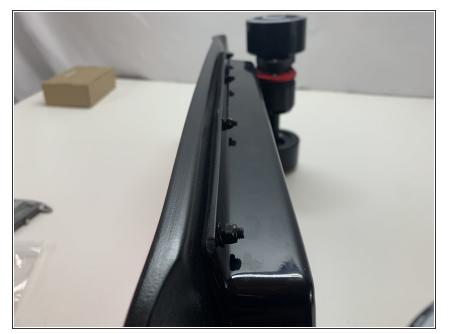
Secure the enclosure with 8x M5x25 bolts, rubber washer, metal washer, and locknut. Make sure the rubber washer is against the enclosure with a metal washer and locknut on top of it.
