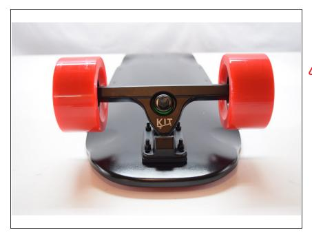
Install the front truck with one riser and 4x M5x35 Bolts and Lock Nuts
