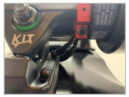
• Align the motor wires so they go through the cable shroud
