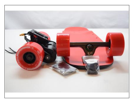
Gather the deck, front truck assembly, drivetrain assembly, 2x risers, and truck hardware.
