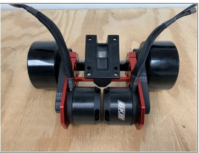
Repeat steps 18-20 to complete assembly of the other side of the drivetrain. Ensure proper belt tension
