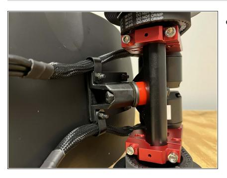
Secure the drivetrain to the deck using 4x locknuts
