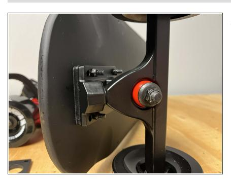
Secure the front truck to the deck with 4x locknuts
