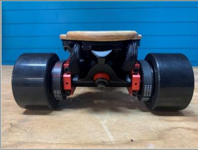
Repeat the previous steps to install the 20T motor pulley on the other side
