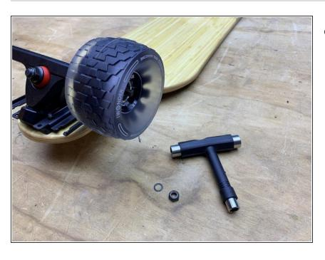
Slide the wheel onto the truck with the white letters facing outwards
